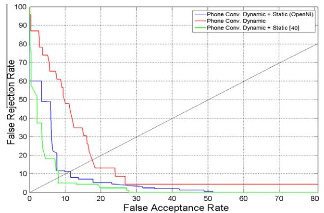
**Fig. 10.** Scenario A – ROC Curves for the fused scores.
