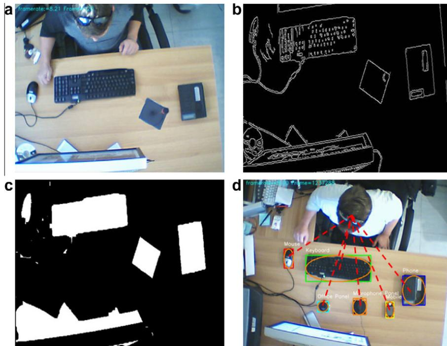
Fig. 8. Object detection: (a) Top camera view, (b) contour extraction (c) objects' area detection, and (d) tagging of objects.
