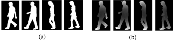
Fig. 2. Illustration of 3-D geodesic transform. (a) Binary silhouettes and (b) corresponding 3-D geodesic distributed silhouettes.
