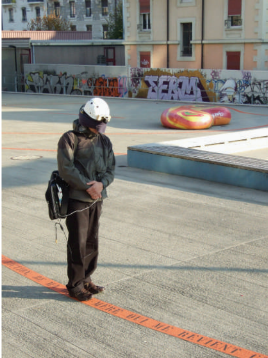
FIGURE 3: A blindfolded experiment participant having a head mounted camera and following a red serpentine line with the See-Color interface. A video showing this experiment is available for download from http://cvml.unige.ch/ .
