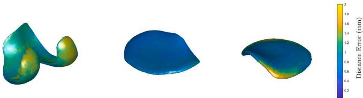
Fig. 15. Spatial distribution of the distance error of the predicted shapes (FC (left), TCM (middle) and TCL (right)) compared to the ground-truth geometries averaged for 15 random subjects in the common space of the mean shape of the PCA-based SSM.
