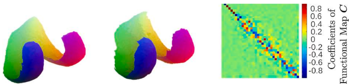
Fig. 3. Correspondence results obtained by the FMNet model on a pair of femoral cartilages. Corresponding points are assigned the same color. (For interpretation of the references to color in this figure legend, the reader is referred to the web version of this article.) The resulting functional map C (right) is sparse and diagonally dominant, indicating that the two shapes are approximately isometric.
