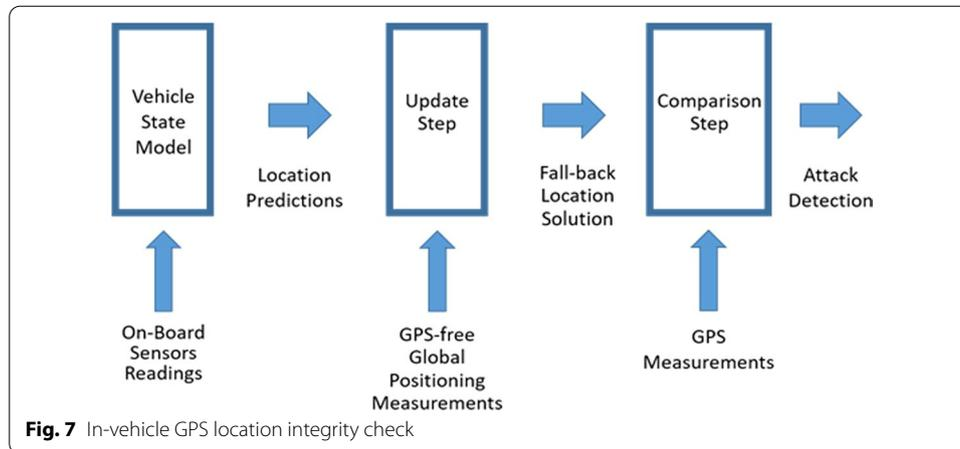
When instead the attack is done from some distance, the relative distance between the attacked GPS receiver and the spoofer needs to be estimated and predicted over short-term time windows. This increases the difficulty of the attack if the actual intent is to alter in an orchestrated way the output of the attacked GPS receiver.
