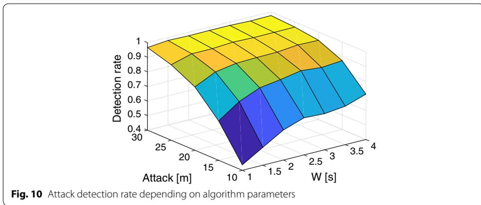
measurements. Nevertheless, the trade-off between the length of the sliding window and the ability of the described attack detection mechanism to quickly react to a GPS spoofing attack has to be taken into account when setting  $W$ .
