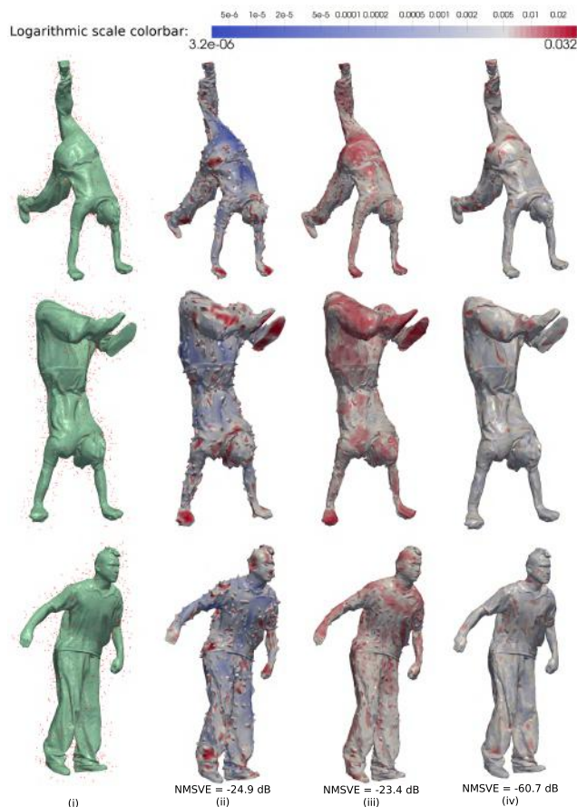
FIGURE 9. Outlier removal on the Handstand animation model: (i) 20% noisy points, (ii) output of WLOP, (iii) output of Static RPCA, (iv) output of RPCA applied to the time-varying point cloud matrix (DRPCA). The proposed outlier removal method successfully identifies and removes the outliers even in the extreme case where 20% of the points can be considered as outliers, randomly distributed over the range of 1/50 of the bounding box’s diagonal length.
