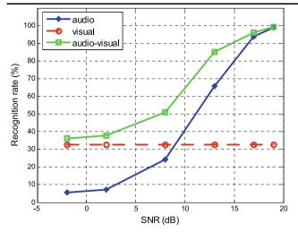
Fig. 7 Word recognition accuracy of the unimodal and the multimodal speech recognition systems at various acoustic noise levels
