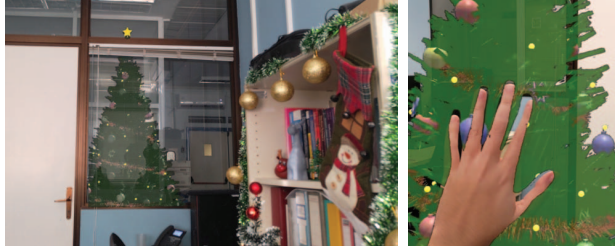
Figure 2: Left: A virtual object behind the glass. Right: A hand model with a black color unlit material tracking the real hand.
