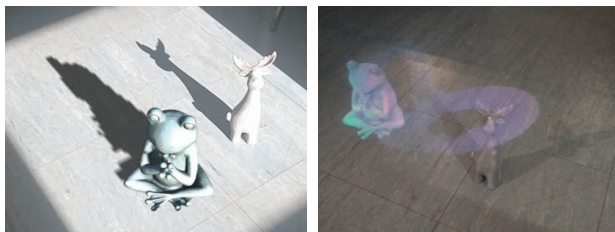
Figure 3: Left: Light estimation based on user’s location, captured with smart device. Right: Virtual and real object comparison with two light sources, captured with HL2.
